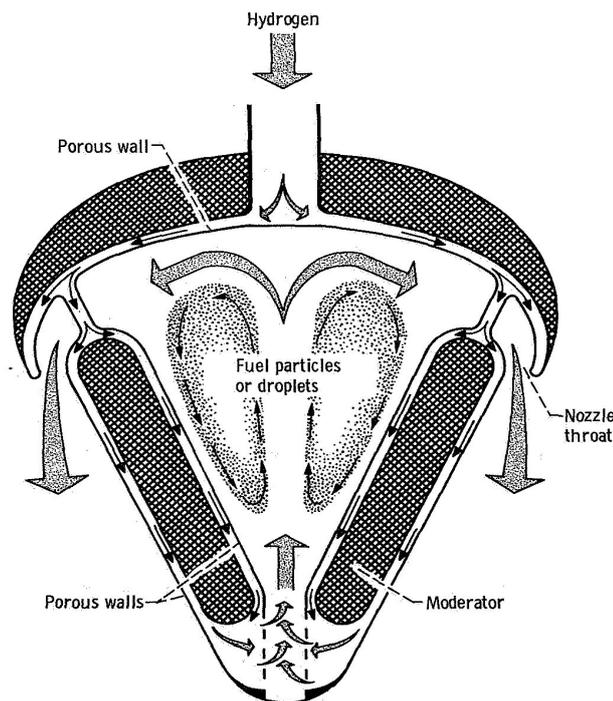
Figure 17 – Drawing of a DLCR propulsion system [R 20]
