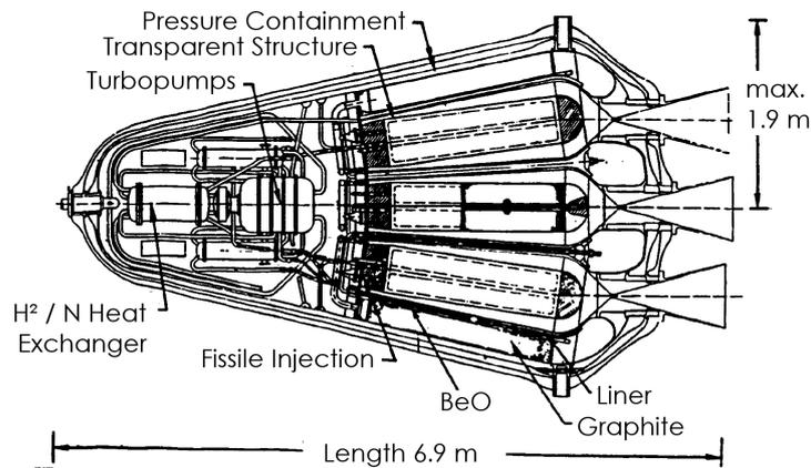
Figure 20 – Cut of a Nuclear Light Bulb Gas Core NTFP
