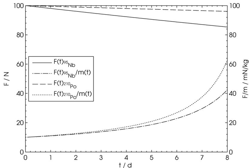
Figure 3 – Exemplary development of thrust and mass specific thrust as a function of time. Isotopes: Niobium 95 and Polonium 210;  $m_0 = 10000$  kg;  $c_e = 8000$  m/s;  $F_0 = 100$  N
