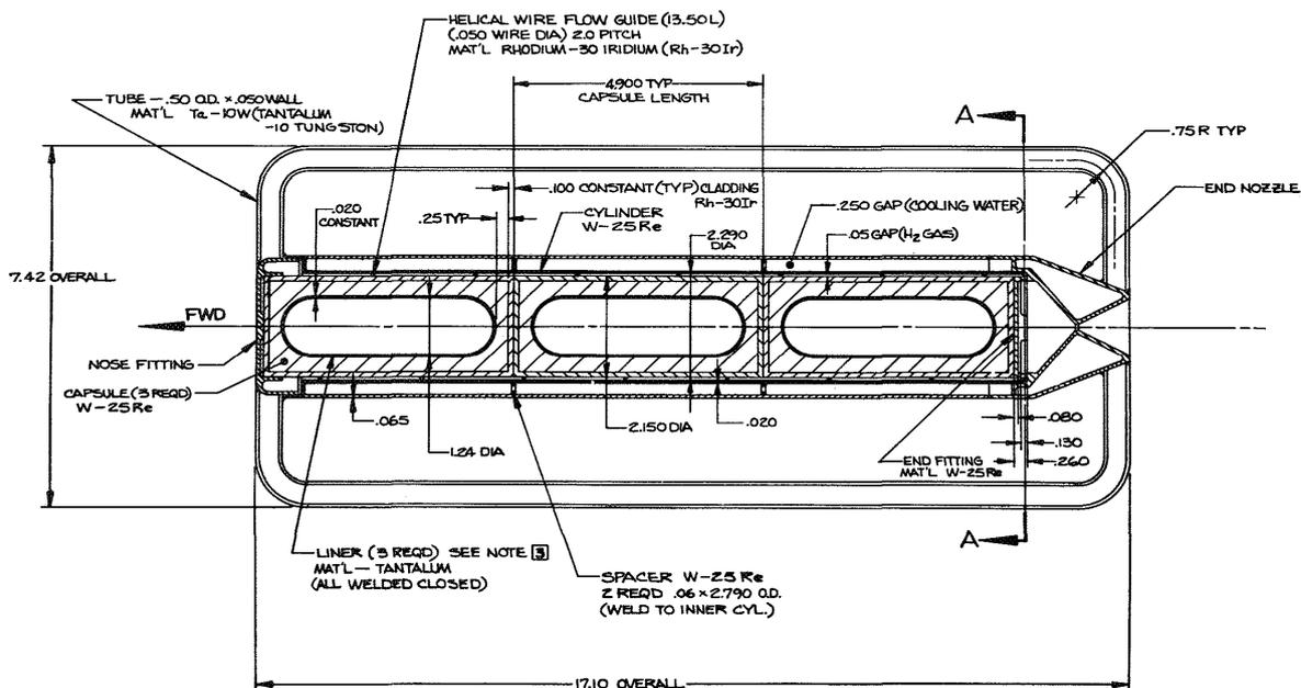
Figure 8 – POODLE drawing from [R 19]. Dimensions in inch (1 inch = 2.54 cm):  $d \approx 0.19$  m;  $l \approx 0.44$  m.
