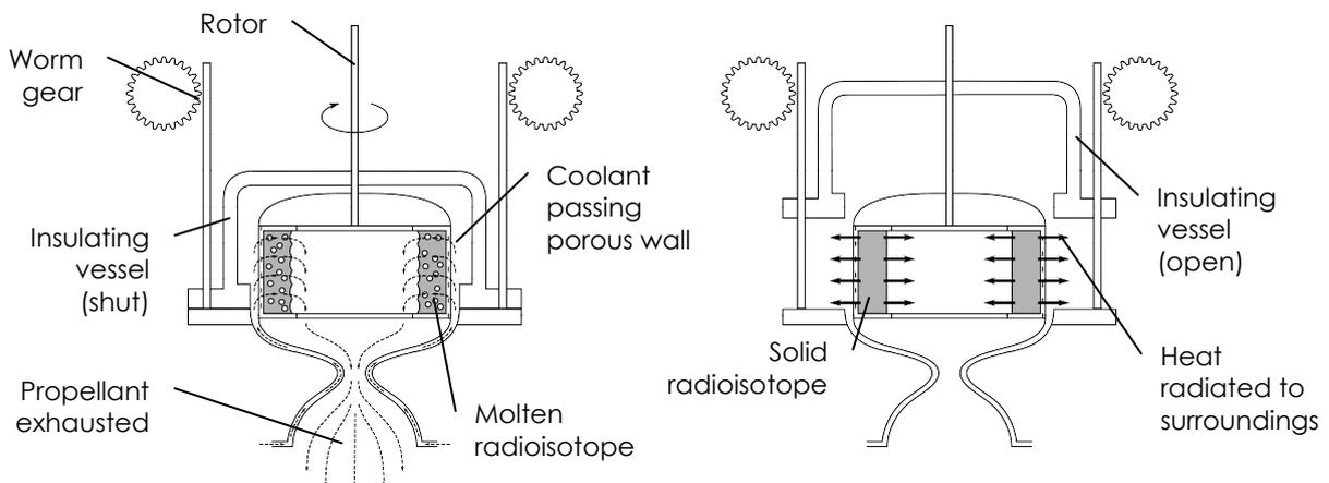
Figure 7 – Schematic draft of a liquid core RHTP [R 16].
