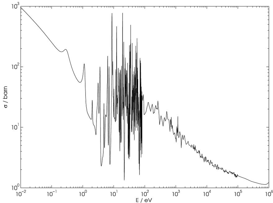
Figure 9 – Fission cross section of <sup>235</sup>U using a neutron as a function of its energy. (1 barn = 10<sup>-28</sup> m<sup>2</sup>) [R 28]
