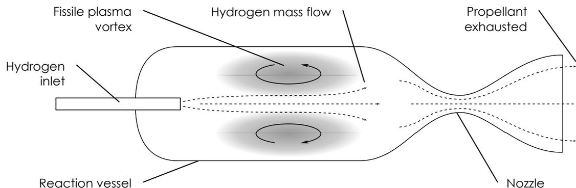
Figure 19 – Schematic draft of a toroidal vortex stabilised Gas Core NTFP
