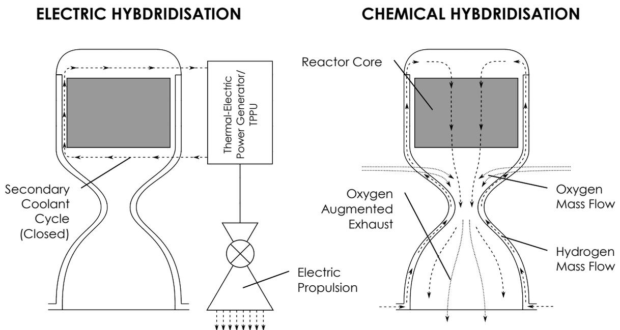
Figure 12 – Hybridisation of solid core NTFP
