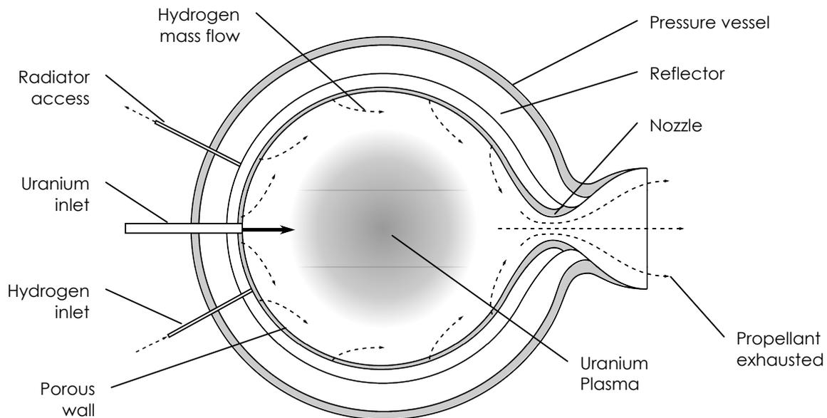
Figure 18 – Schematic draft of a generic Gas Core NTFP
