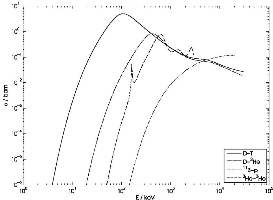
Figure 24 – Fusion cross sections
