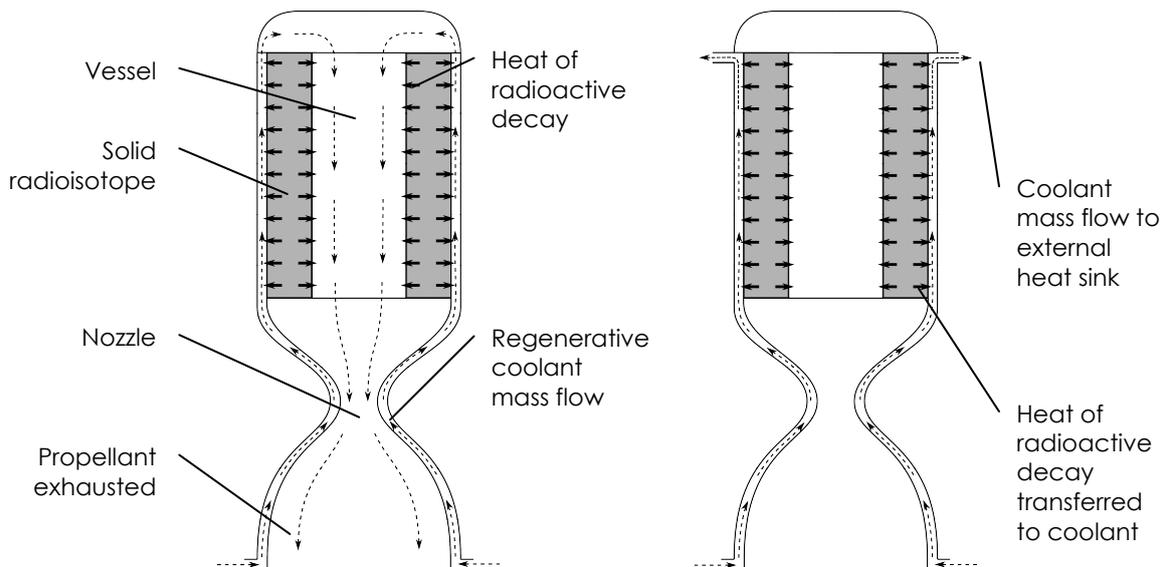
Figure 5 – Schematic draft of a solid core RHTP with active cooling in idle mode [R 16].
