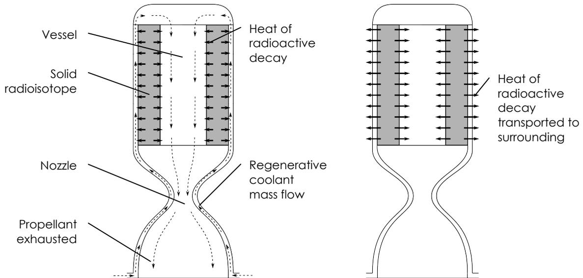
Figure 4 – Schematic draft of a solid core RHTP with passive cooling in idle mode.
