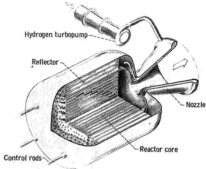
Figure 10 – Schematic view of a generic heterogeneous solid core NTFP [R 20]
