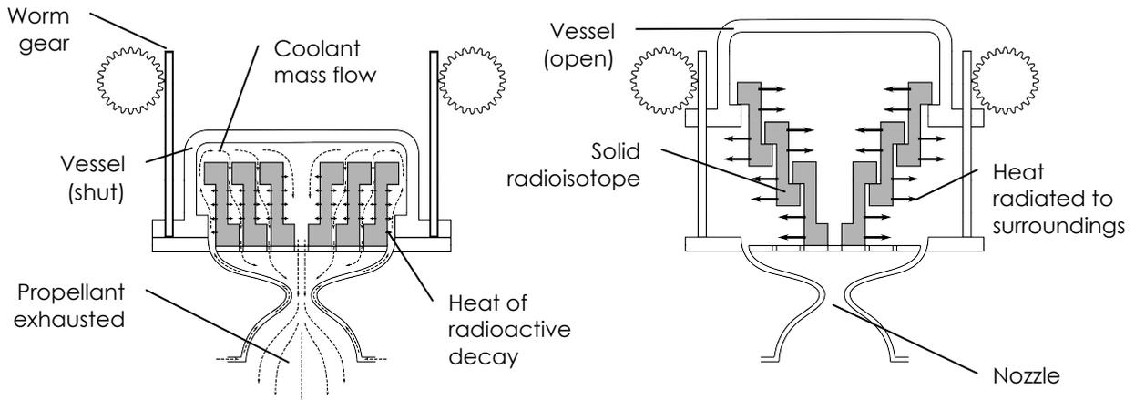
Figure 6 – Schematic of a solid core RHTP with extended core in idle mode [R 16].
