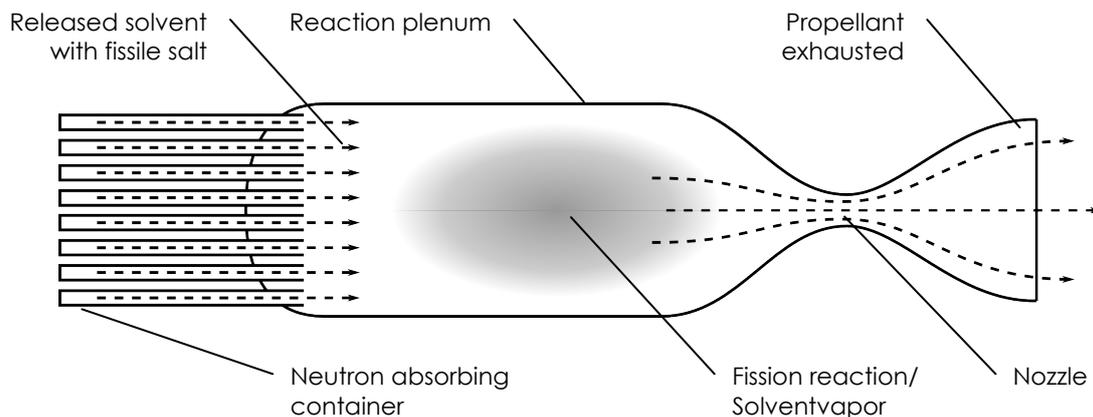
Figure 22 – Schematic draft of a NSWR.
