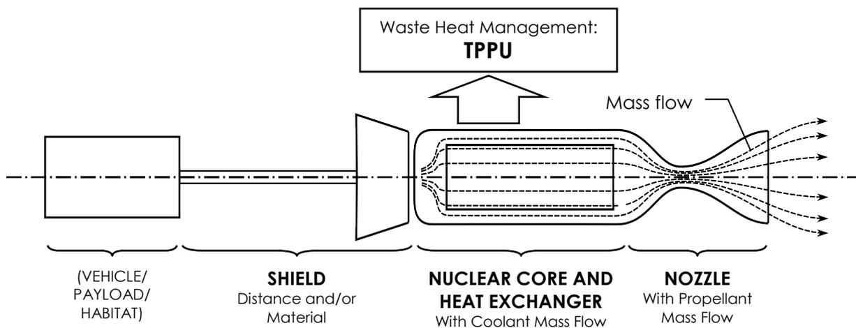
Figure 2 – Schematic presentation of Nuclear Thermal Propulsion Systems.
