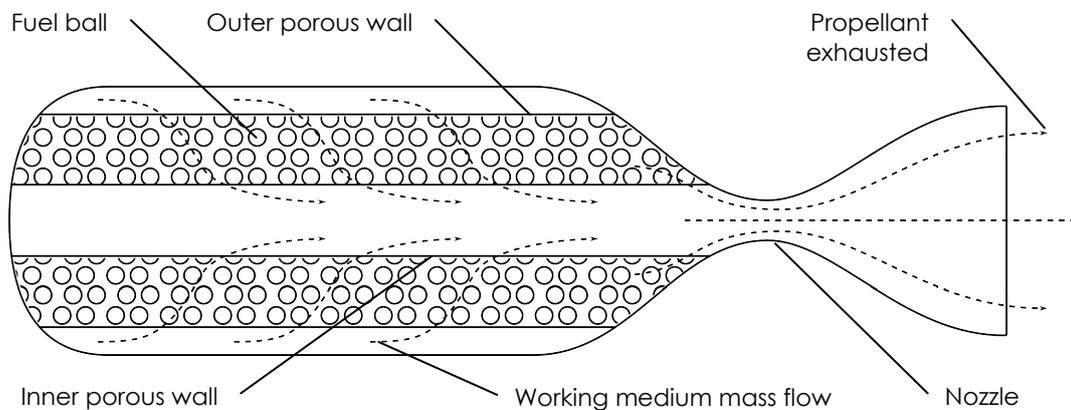
Figure 11 – Schematic draft of a pebble bed NTFP
