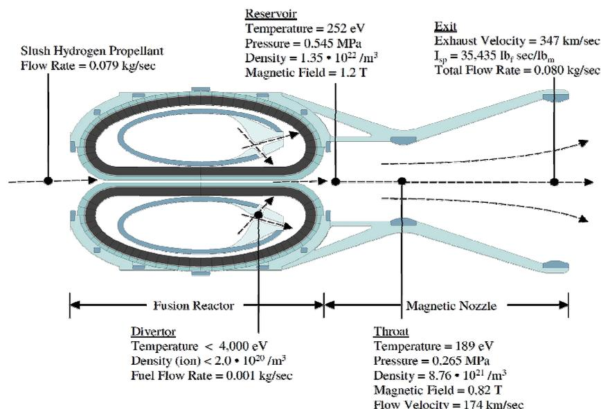
Figure 26 – Fusion NTFP according [R 58]
