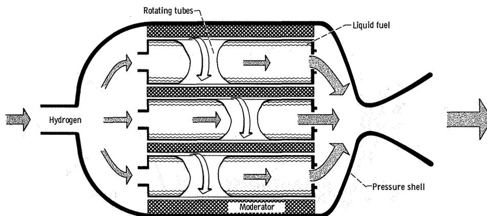
Figure 16 – Drawing of a rotationally stabilized backflow free Liquid Core Reactor NTFP system [R 20]
