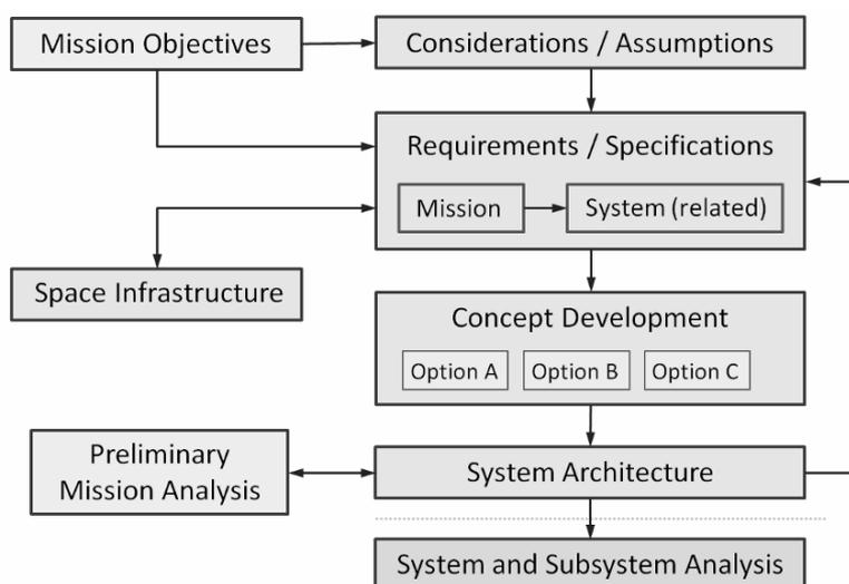
Figure 5 – Simplified evaluation flow diagram of space vehicle.
