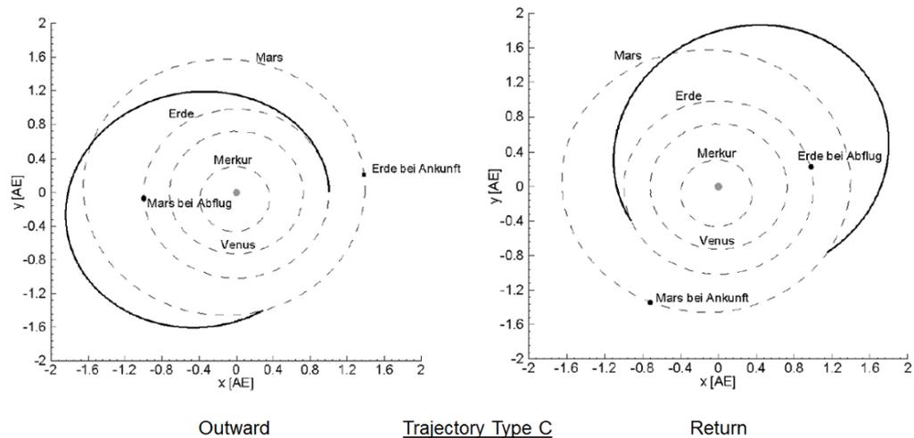
Figure 9 – Schematic view of C-type trajectory from orbit 0 to orbit 1 (Earth-Mars orbit transfer) [R 38].
