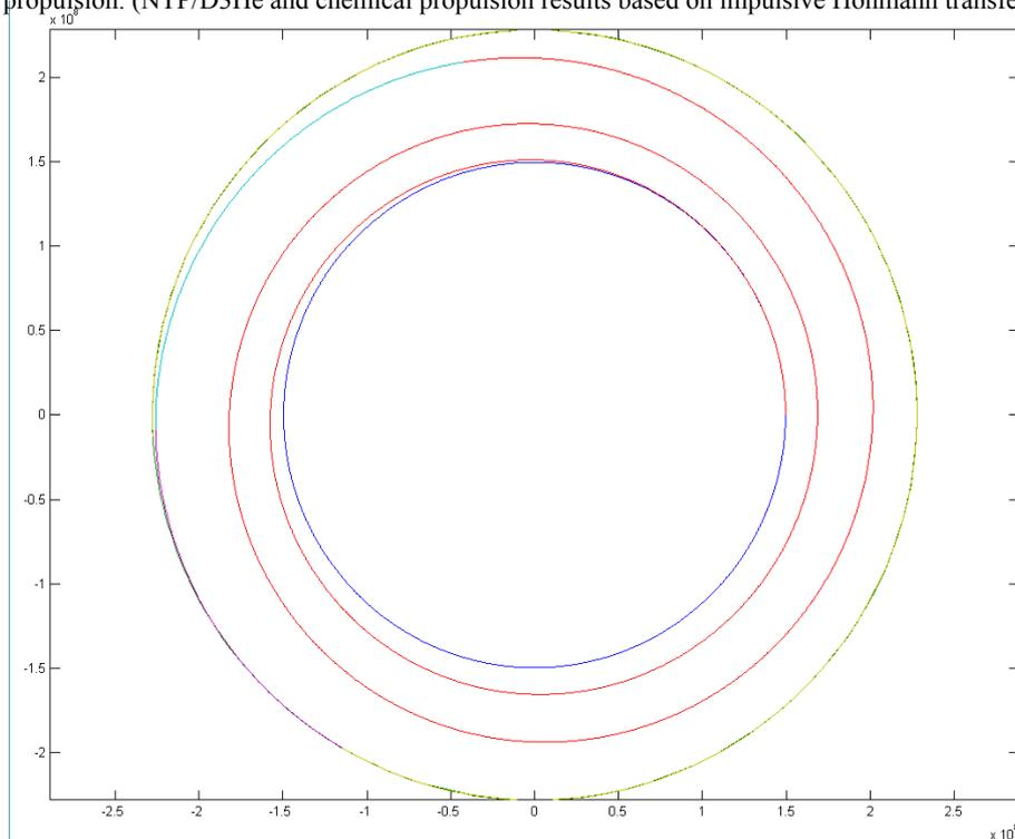
Figure 17 – Trajectory of Mars I mission scenario with HiPARC NEP and power density of 20 W/kg (150 t initial mass and 100 t payload mass).
