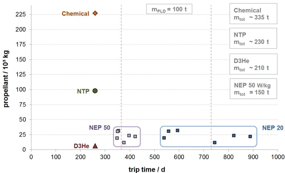
Figure 16 – Comparison of analysis results of Mars I mission scenario with NEP / NTP / NFTP concept and chemical propulsion. (NTP/D3He and chemical propulsion results based on impulsive Hohmann transfer).
