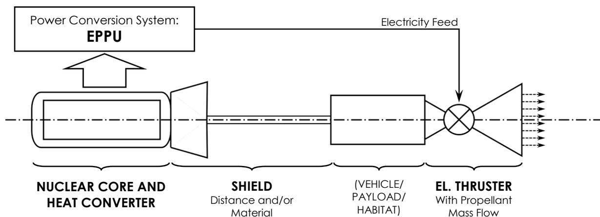
Figure 3 – Schematic presentation of generic fission based Nuclear Electric Propulsion Systems.
