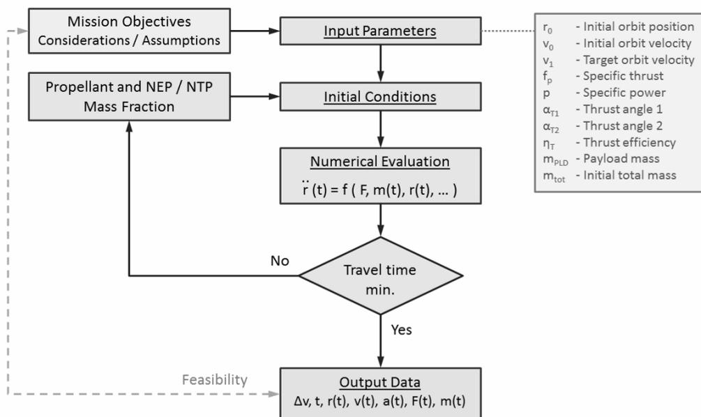
Figure 13 – Flowchart of MATLAB mission analysis tool.
