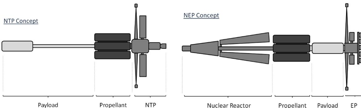
Figure 6 – Mass related system architecture of NTP and NEP based space vehicle concepts.
