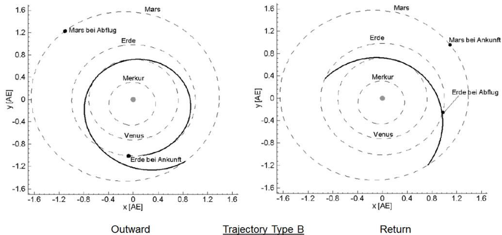
Figure 8 – Schematic view of B-type trajectory from orbit 0 to orbit 1 (Earth-Mars orbit transfer) [R 38].
