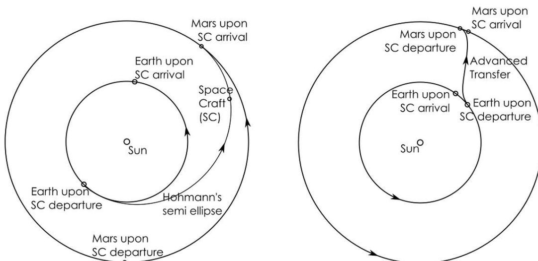
Figure 4 – Schematic of Hohmann's transfer (left) and the continuous-burn-rendez-vous (right).
