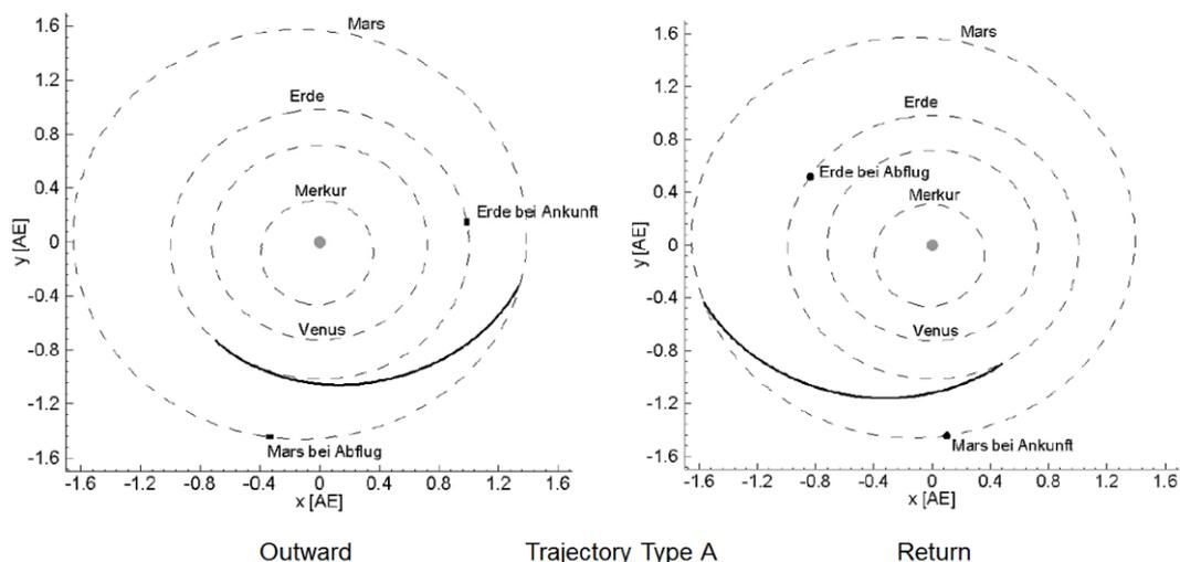
Figure 7 – Schematic view of A-type trajectory from orbit 0 to orbit 1 (Earth-Mars orbit transfer) [R 38].
