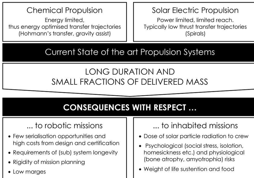
Figure 1– Current state of the art propulsion features and consequences overview.
