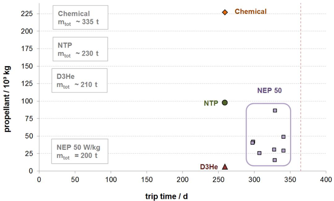
Figure 20 – Comparison of analysis results of Mars II mission scenario with NEP / NTP / NFTP concept and chemical propulsion. (NTP / NFTP and chemical propulsion results based on impulsive Hohmann transfer).
