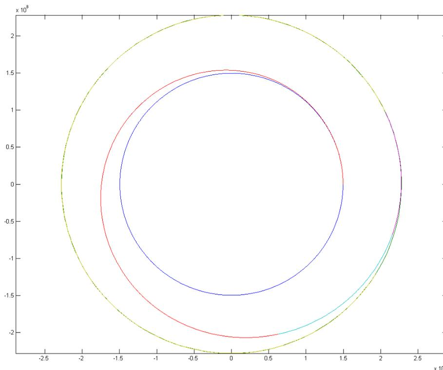
Figure 18 – Trajectory of Mars I mission scenario with NEXT NEP and power density of 20 W/kg (150 t initial mass and 100 t payload mass).
