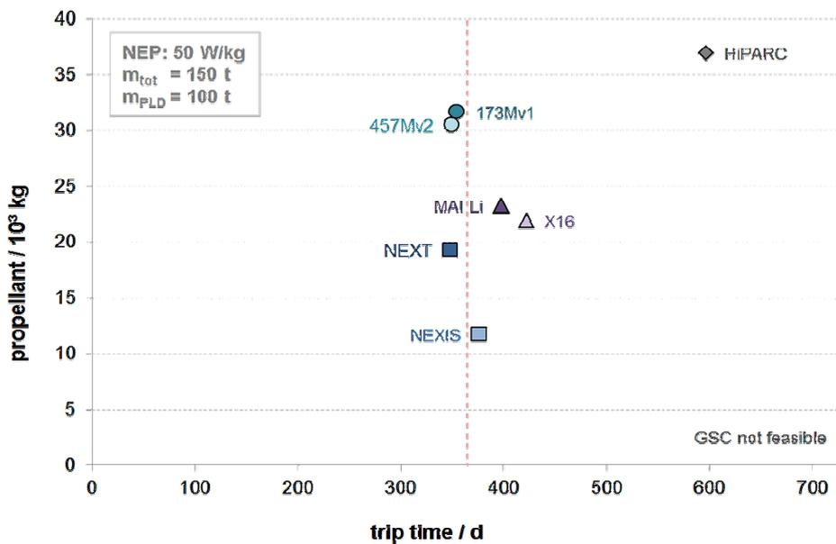
Figure 15 – Analysis results of Mars I mission scenario with NEP concept for specific EP system and power density of 50 W/kg for nuclear power (150 t initial mass and 100 t payload mass).
