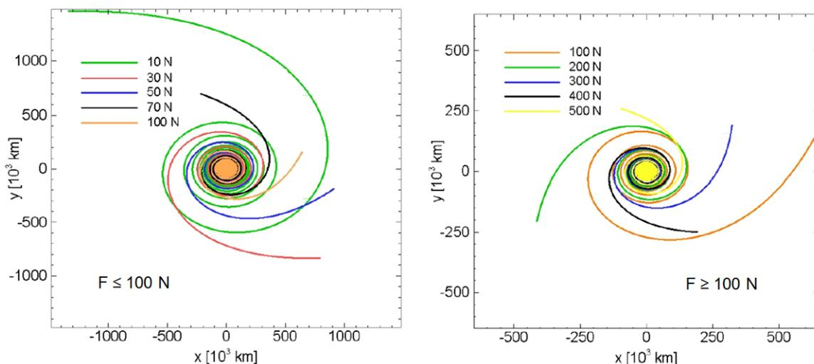
Figure 11 – Trajectories at different thrust levels and respective specific impulse of 3000 s [R 38].
