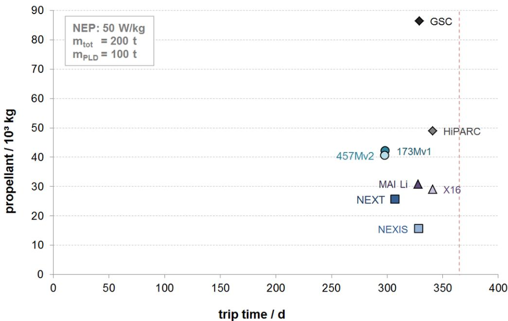
Figure 19 – Analysis results of Mars II mission scenario with NEP concept for specific EP system and power density of 50 W/kg for nuclear power (200 t initial mass and 100 t payload mass).
