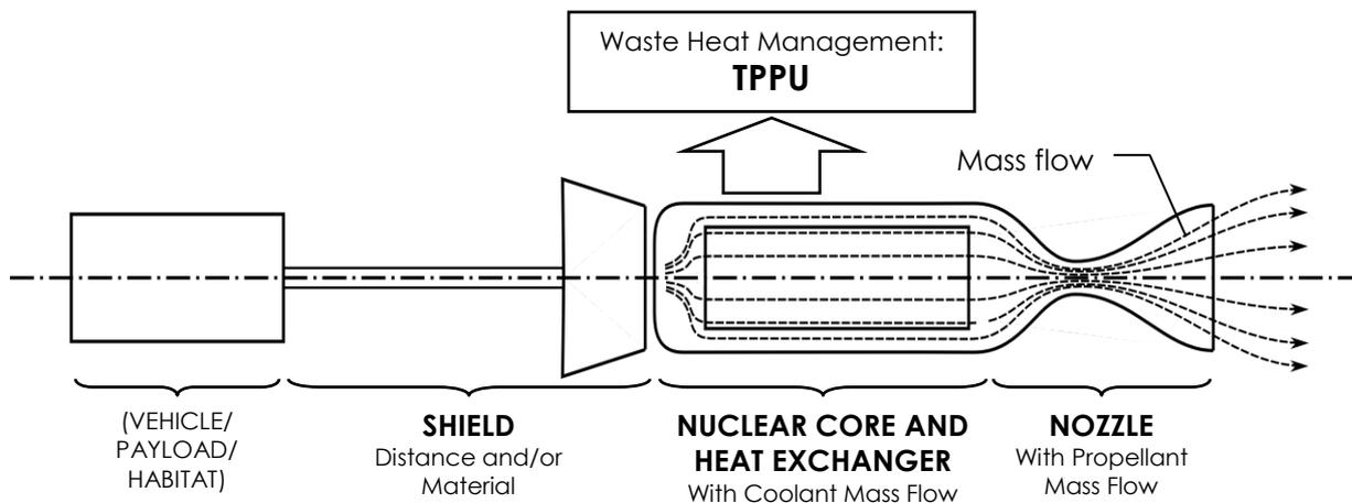
Figure 2 – Schematic presentation of Nuclear Thermal Propulsion Systems.
