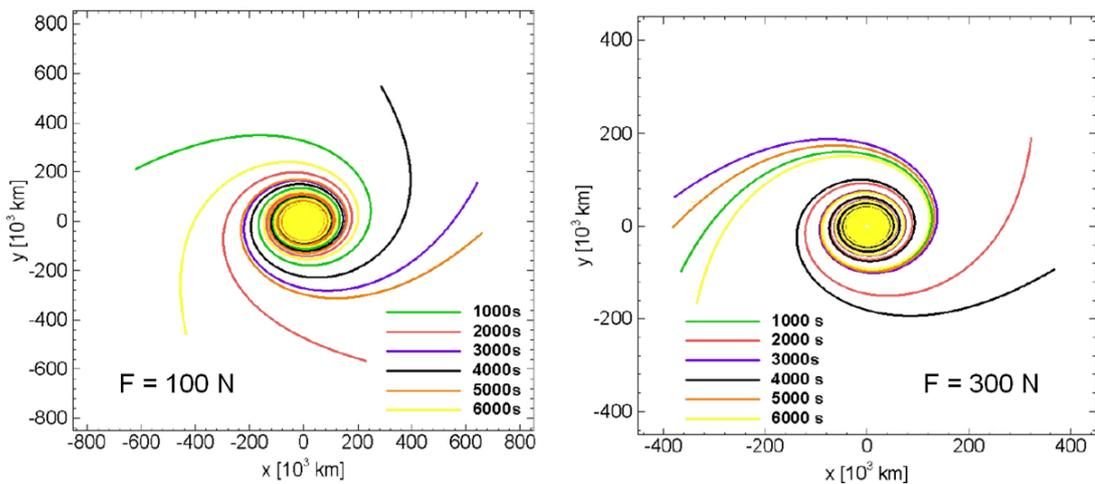
Figure 12 – Trajectories at different specific impulse levels and respective thrusts of 100 / 300 N [R 38]
