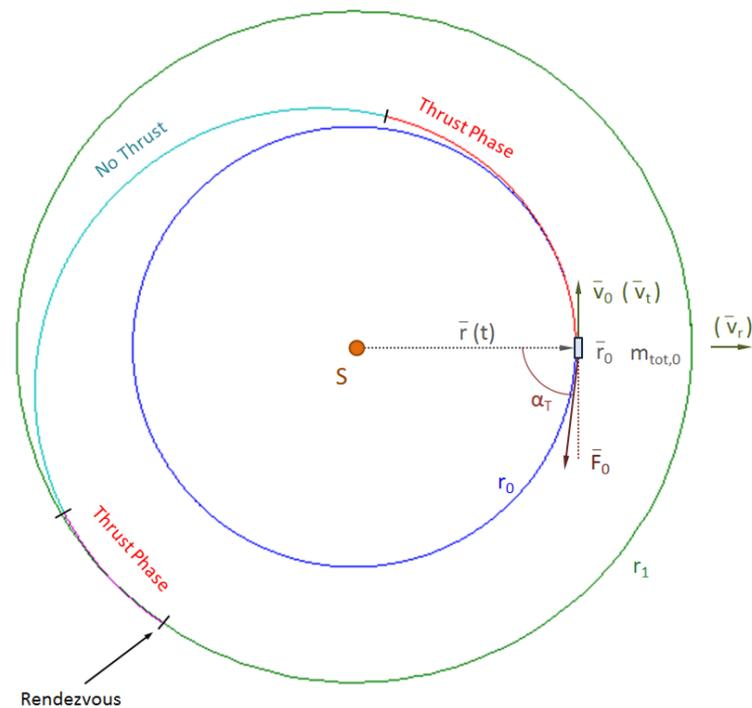
Figure 10 – Schematic view of trajectory from orbit 0 to orbit 1 evaluated by MATLAB mission analysis tool.
