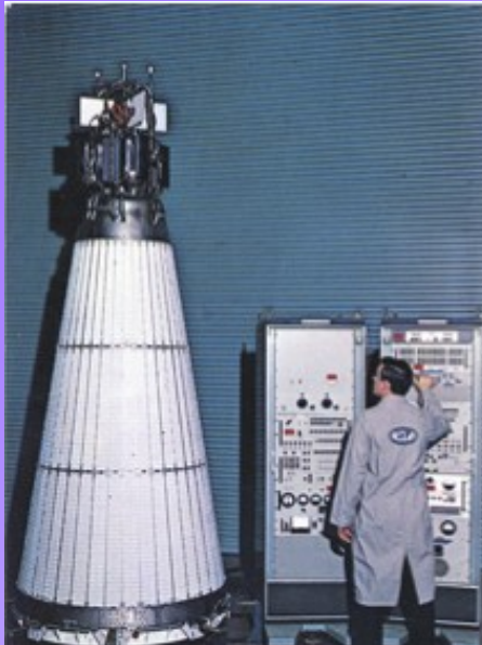
The Romashka NPS reactor converter layout: (1) radiator ribs, (2) thermoelectric elements, (3) control rod, (4) reactor vessel, (5) upper reflector, (6) reactor core, (7) radial reflector. Source: Kurchatov Institute.
