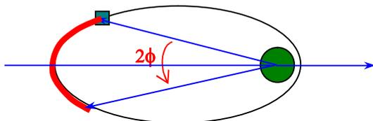
Example of **thrust arc** centred around the apogee with a true anomaly amplitude of  $2\phi$ .
