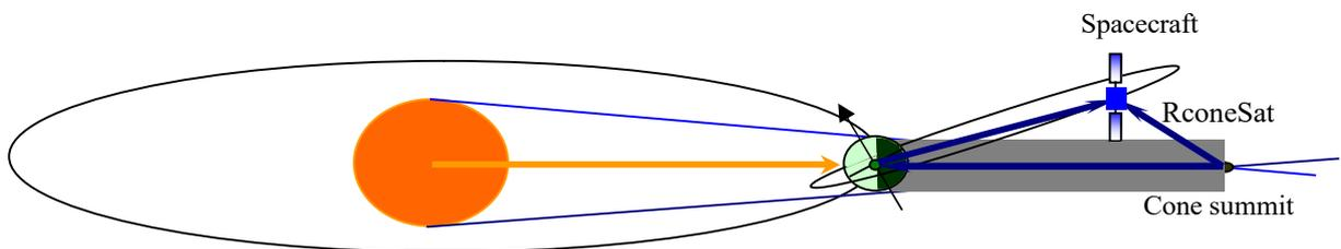
Example of the configuration Sun, Earth , shadow cone summit and Earth Spacecraft on an elliptical orbit.
