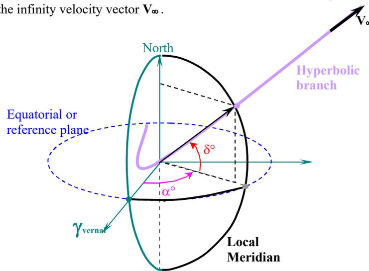
Note : For a travel from planet to planet, roughly, the lowest cost trajectory in terms of delta V constrains the declination with the date of the travel:
