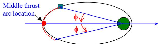
Specification of the same **thrust arc** in TriaXOrbital: half-thrust arc =  $\phi$ , and the middle thrust arc location at apogee.
