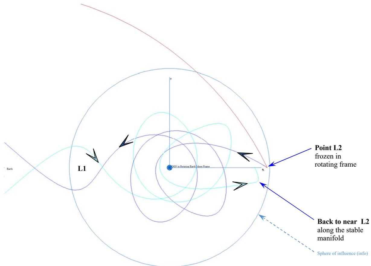
Figure 7: ZOOM of TriaXOrbital plot at L2 in the rotating frame: diverging L2 and converging back again near L2
