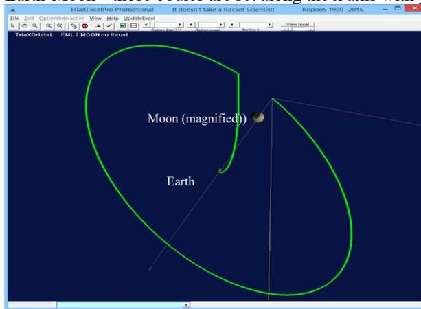
Figure 1: 3D view (under TriaXExcelPro) of the two impulses Transfer Trajectory followed by a stay at L2 for one Moon period, in ECI
