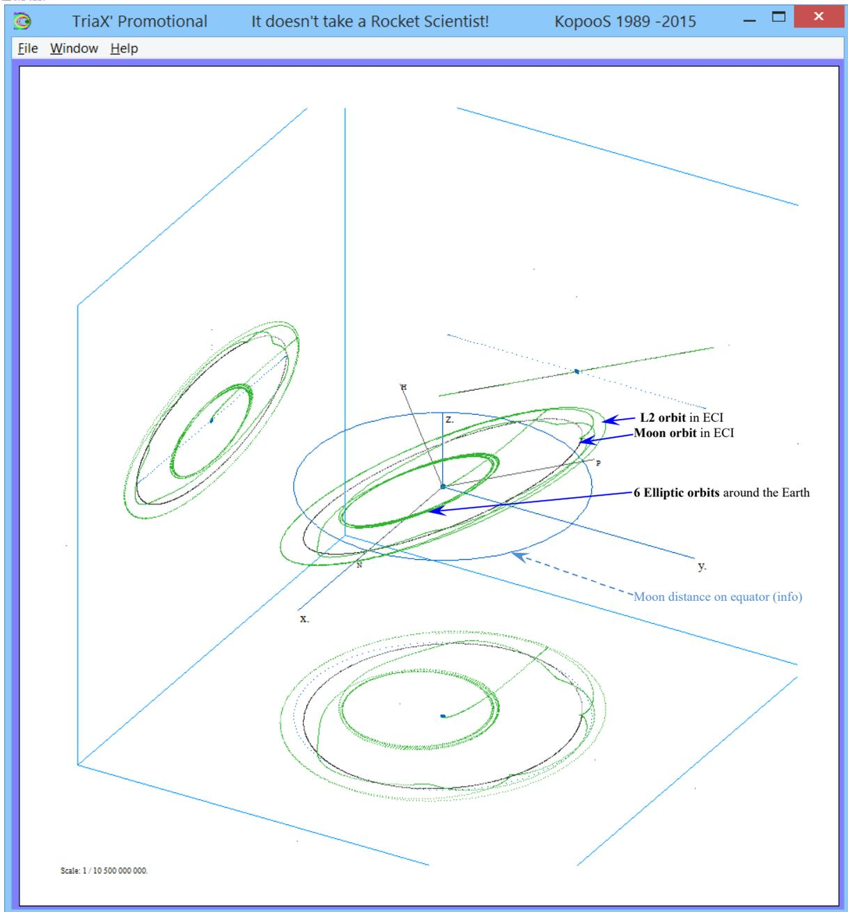
Figure 8: TriaXOrbitaL plot (from a two impulses Transfer followed by a stay at L2 for 30 days) diverging L2 in ECI
