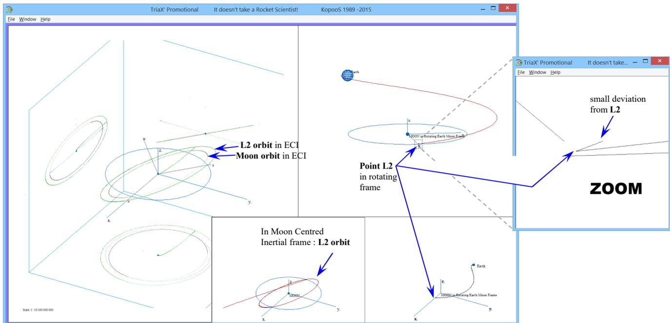
Figure 2: Orbits of L2 in ECI, in Moon Centred Inertial and Point L2 in the rotating synodic E-M frame
