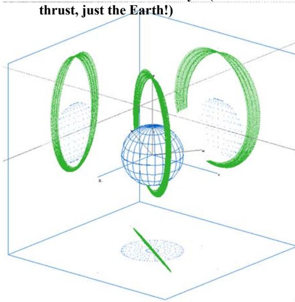
**Classical orbit transfer (thrust 500 N) : 3 thrust arcs**
