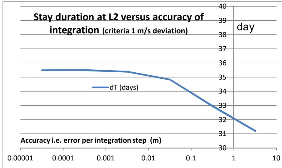
Figure 3: Evolution of the duration at L2 before deviation occurs versus integration errors levels
