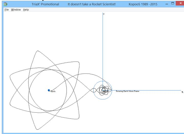
Figure 6: TriaXOrbital plot (from a two impulses Transfer followed by a stay at L2 for 30 days) diverging from and converging again back to near L2
