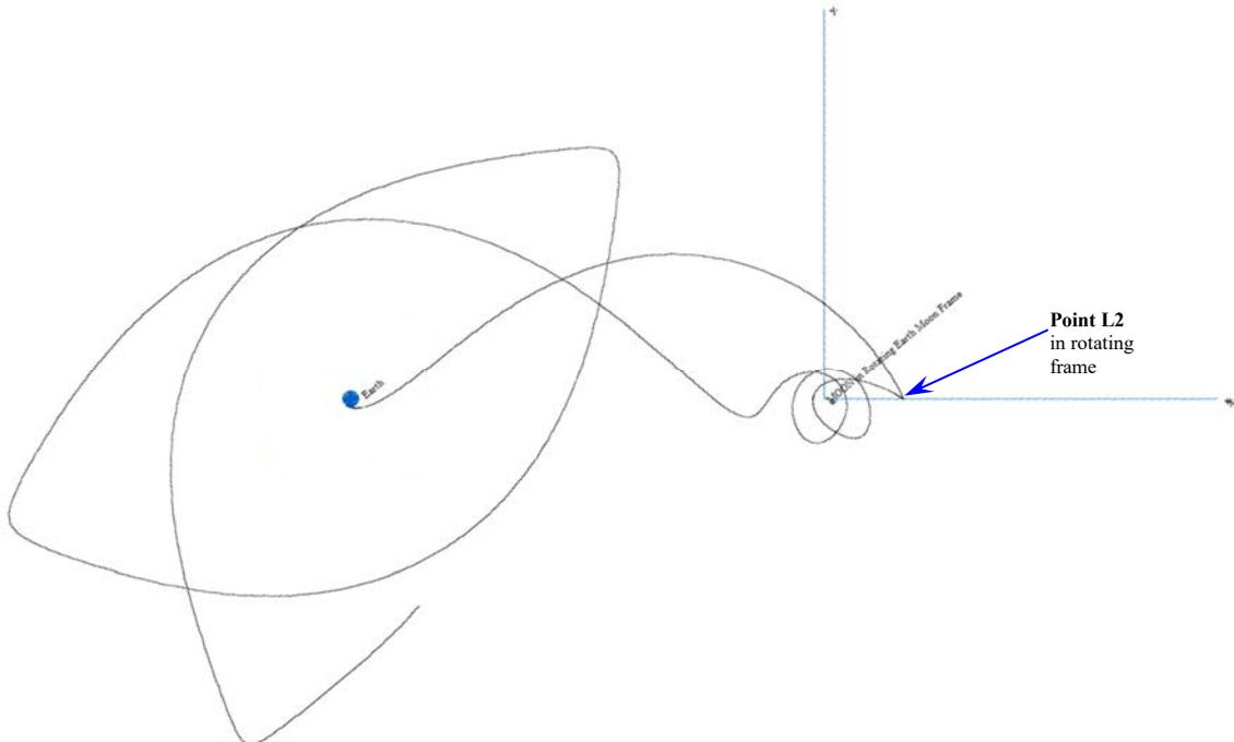
Figure 5: TriaXOrbital plot (starting from a two impulses Transfer Trajectory followed by a stay at L2 for 30 days) and diverging L2 on the unstable quasi-invariant manifold
